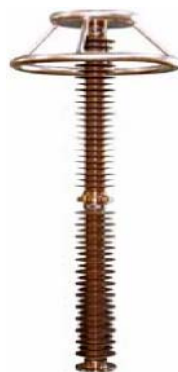
198kV polymeric arrester with 40kA pressure relief
